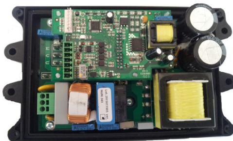
Fig. 2 – DDMP 1kW Driver – Complete view
