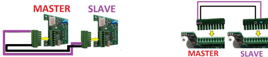
Fig. 12 – MASTER/SLAVE connection 0-10V
