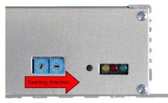
Figure 13: Fan Controller Address Switches
