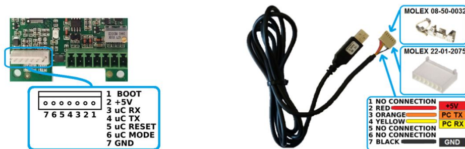
Fig.38 – White OFFLINE connector and OFF line Cable
